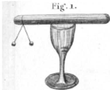
Detail of similar experiment using cork balls suspended from an insulated conductor.
