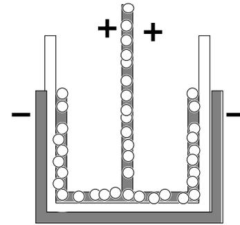
Here the Leyden jar has all of the normal amount of electrical fire that was on the outer coating transferred to the inner coating. I have not drawn the 20 plus signs and 20 minus signs that should appear
