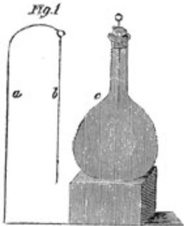
Here is Franklin's illustration of this experiment reproduced from the plate in Bigelow, plate III Vol II, p. 200
