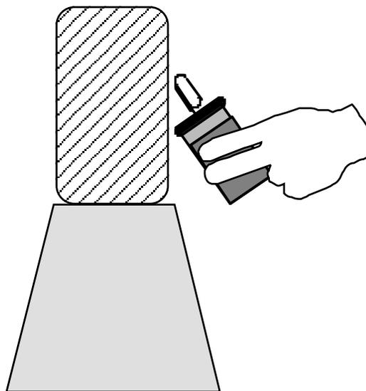
The diagram above shows electrification of a soda can repeatedly from the wire of the Leyden jar. Test for charge with the neon bulb.
