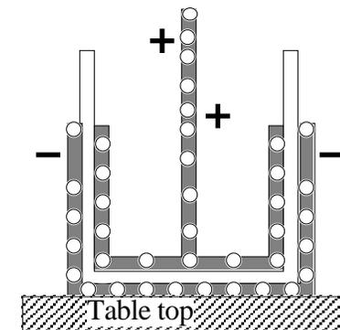
In the lower diagram two parts of the 20 in the outer coating have been moved to the inner coating, marked by +, since it now has an extra quantity of electricity. The outer coating, having lost electricity, has less than its normal quantity marked by -.
