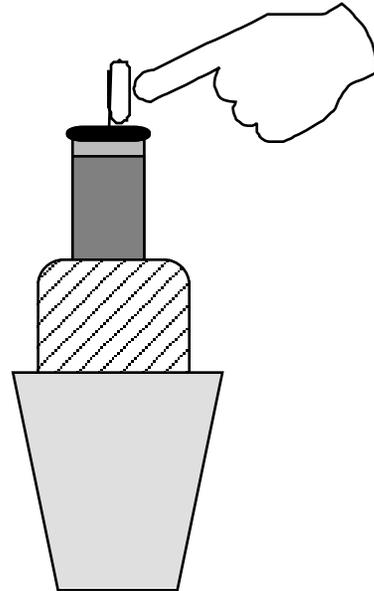
Set the charged Leyden jar down on the first soda can and touch the wire. Then lift it by the wire and set it on a foam cup. Pick it up by the coating and touch the wire to the other soda can.
