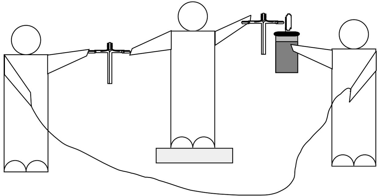
You can do this experiment full size using people, and use the neon bulbs to monitor the direction of discharge, as shown in the diagram.
