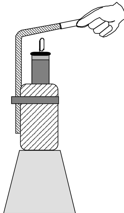
The diagram at right shows the attempt to electrify the soda can from the wire of the Leyden jar that rests on top of the can. Bend the foil covered straw down to touch the paper clip, holding only onto the uncovered part. Test the can for charge with the neon bulb, then test the Leyden jar for charge with the neon bulb.
