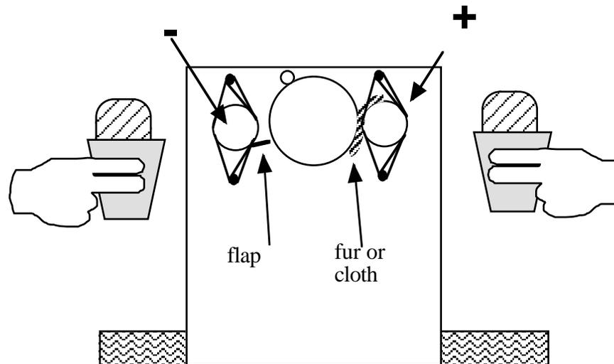
Your generator is built to charge PLUS at the rubbing terminal and to charge MINUS at the collecting terminal. Charge two soda cans in foam cups, one plus and one minus. Have a third soda can in a foam cup. Touch it with your finger to be sure it is neutral or in the 'common state'.
