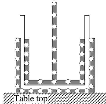
The diagram shows a cross-section of a Leyden jar, with 20 circles to represent the normal electric matter in each.
